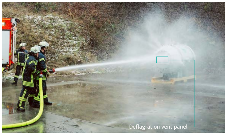
Figure 11: BESS.TGV maintaining full integrity under severe fire hose impact.
