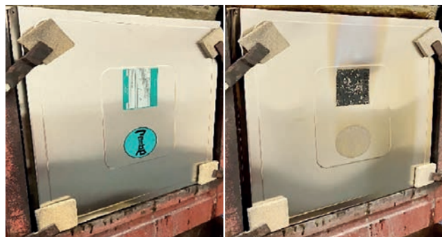
Figure 10: BESS.IKLIEGV maintaining full integrity in furnace test. Sample shown prior to test (left) and after 120 min at 1050 °C furnace peak temperature (right).
