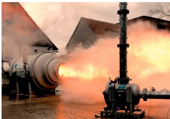
Figure 9: Explosion testing under controlled conditions to validate protection design, performed at REMBE® Research+Technology Center.
